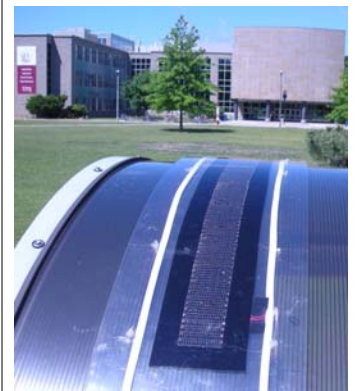
Exterior view of flexible solar strip designed by engineering researchers at McMaster on curved bus shelter. Credit: McMaster University
